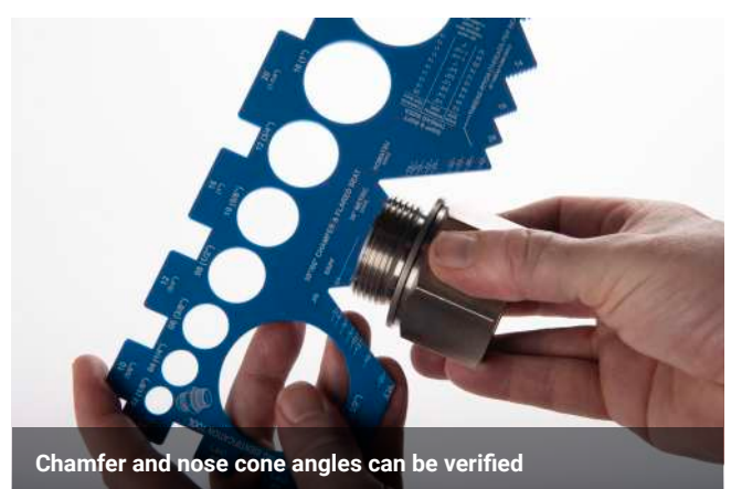
Ports are used to identify male threads, posts for female threads
